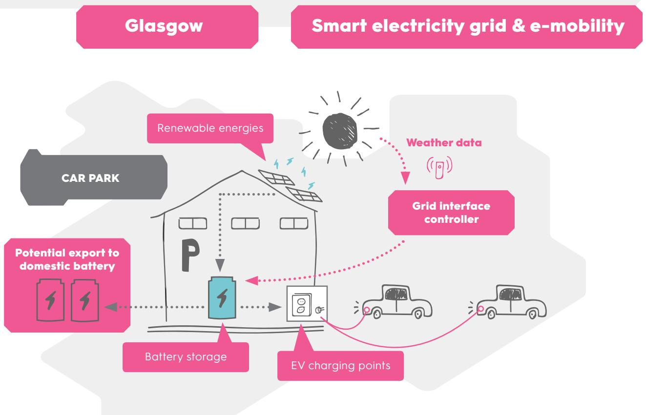
These solutions represent a technological and business case challenge linked to the physical deployment and connection of onsite battery storage, as well as understanding how energy is purchased from local generators, supplied to the battery, and sold by the storage provider either to local points of consumption or to provide grid balancing services.
