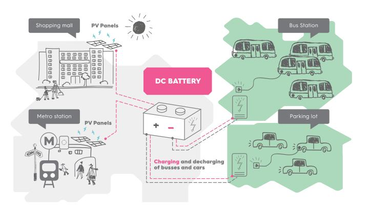
The aim of this smart solution is to minimise and optimise the usage of electricity and avoid peak load demands in the electrical network, by using photovoltaic (PV) panels. Private electric cars that are parked in parking spaces in the Heart of South district will then be able to charge with electricity coming from the PV panels connected to charging poles through an electric direct current (DC) grid.
